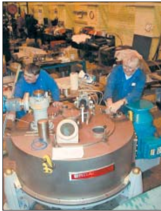
Converting hydraulic drive to electric drive and plough on a fully refurbished Broadbent batch centrifuge and incorporating the latest design features to give the benefits only expected from new equipment
