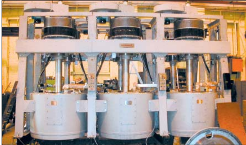
Typical refurbishment of six 25 year old sugar batch centrifugals
