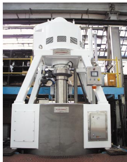
Figure 2. A modern 1300 Kg batch centrifugal with 3 speed motor and DC braking.
