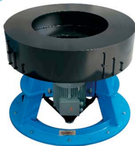
(4) - Test environment 2: 2.2m diameter, 880g-tonne drum
