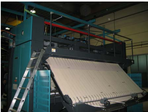
The top section of the machine is easy accessible by standard stairs and service bridge.
