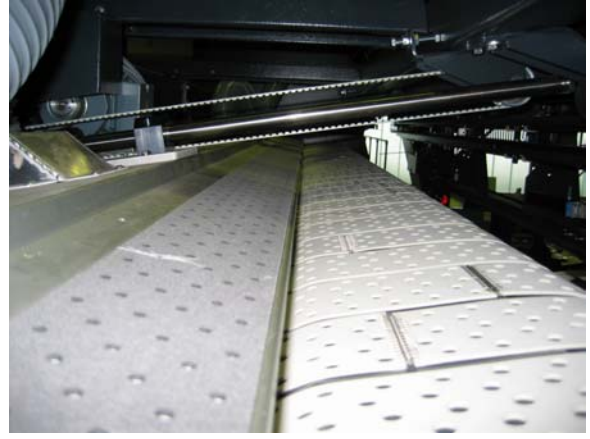
Feeding beam with high vacuum and vacuum under transport belts to secure quality lay down. Maintenance free beam guiding.
