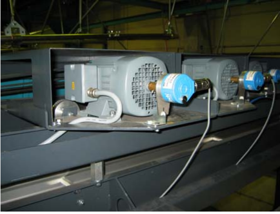
Accurate positioning of clamps by servo control.
