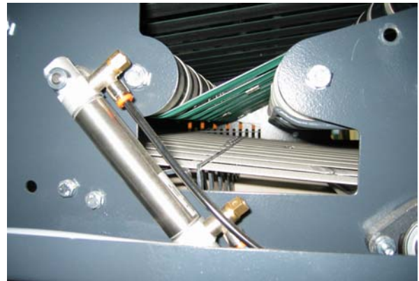
Crossfold with knife upwards with flexible belts can be used as 2 nd or 3 rd crossfold
