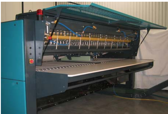
The fold sections are easy accessible by use of a turnable cover.
