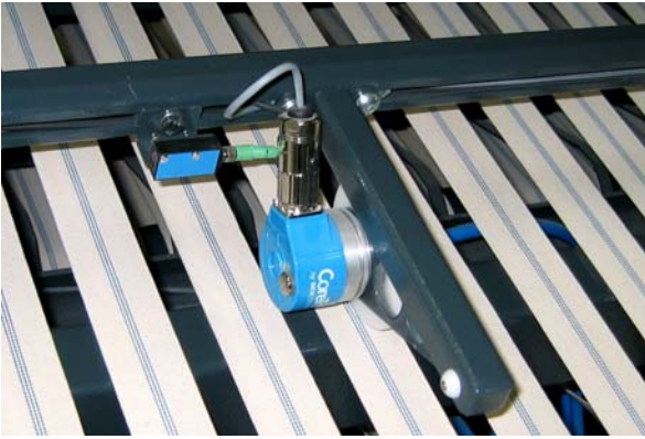
Folding measurement by robust encoder.
