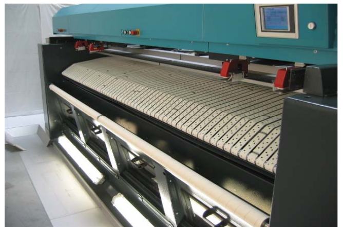
Multilane manual feeding onto belts with vacuumbox
