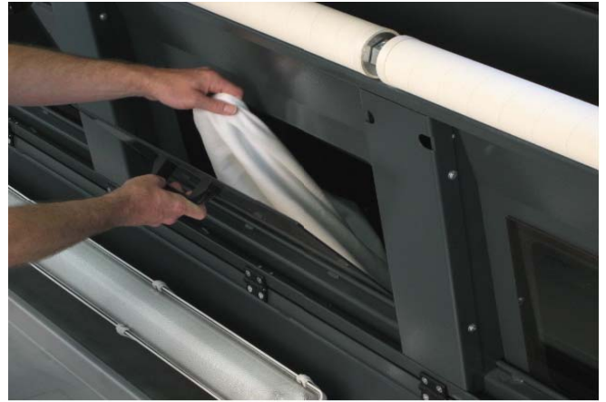
• Easy to remove sheets out of suctionbox
