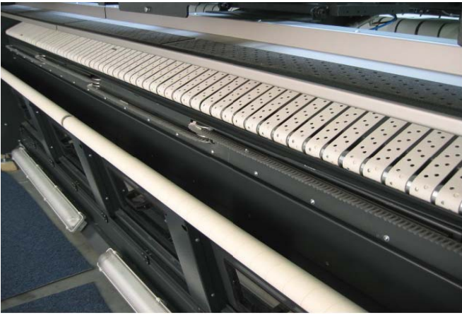
Spreading brushes and knife in suctionbox
